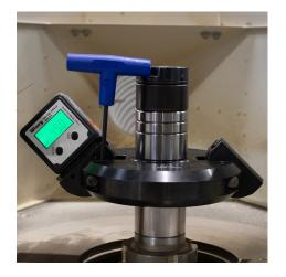
**3.** Use an Allen key to unlock the jaw and rotate it to the required angle, then lock it into position. For the other side, rotate the head and repeat the process.
