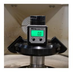
1. With the Vari Angle Head on the shaft, slide the digital protractor onto the flat body of the cutter head, positioning it centrally.
