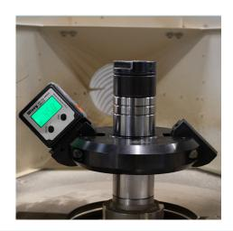
2. Press the button on the digital protractor to reset it to '0'. Remove the protractor from the body and place it on the edge of the cutting jaw.
